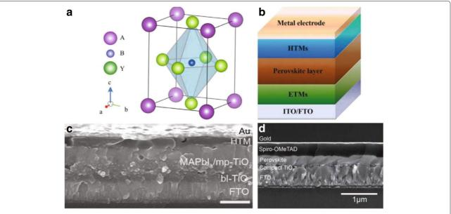
Fig. 2 a Crystal structure of a perovskite [22]. b Schematic diagram of general device [23]. c Cross-section scanning electron microscopy (SEM) images of a meso-superstructured perovskite solar cell (scale bar is 500 nm) [22]. d Cross-section SEM images of a normal planar perovskite solar cells with the presence of an HTL and an ETL [22]
