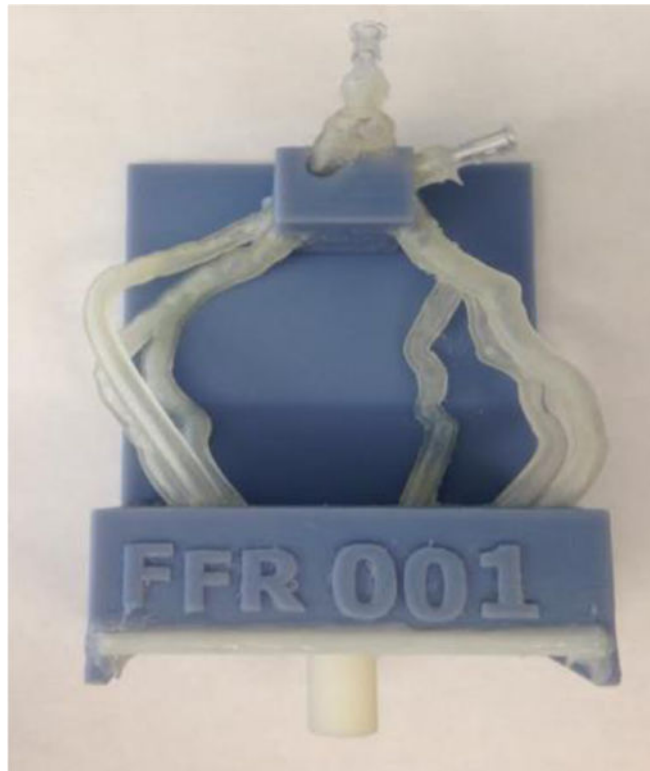
Figure 5. Patient-specific 3D printed coronary arteries used to collect FFR data. The reservoir door and Cole Parmer luers are attached for controlled flow and pressure data.
