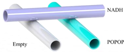
Fig. 4. Schematic of the stacked capillary model. The top purple tube represents NADH/FAD and the bottom teal tube represents POPOP.
