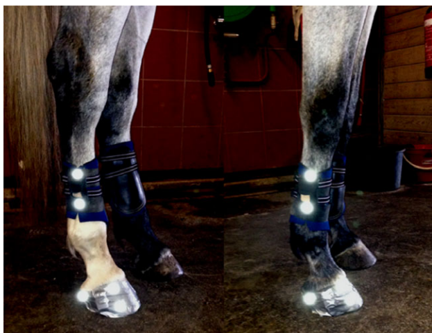
Fig 1: Reflective motion capture markers and inertial measurement unit (IMU) sensors attached to a horse in standardised locations. The IMU sensors were attached to the right lateral metatarsal and metacarpal bones, one reflective marker was placed above and beneath each sensor. Also, three markers were attached to the right fore- and right hind hooves (heel, lateral toe and lateral coronet), but only the lateral heel and lateral toe markers were used for the motion capture detection algorithm in the current study.
