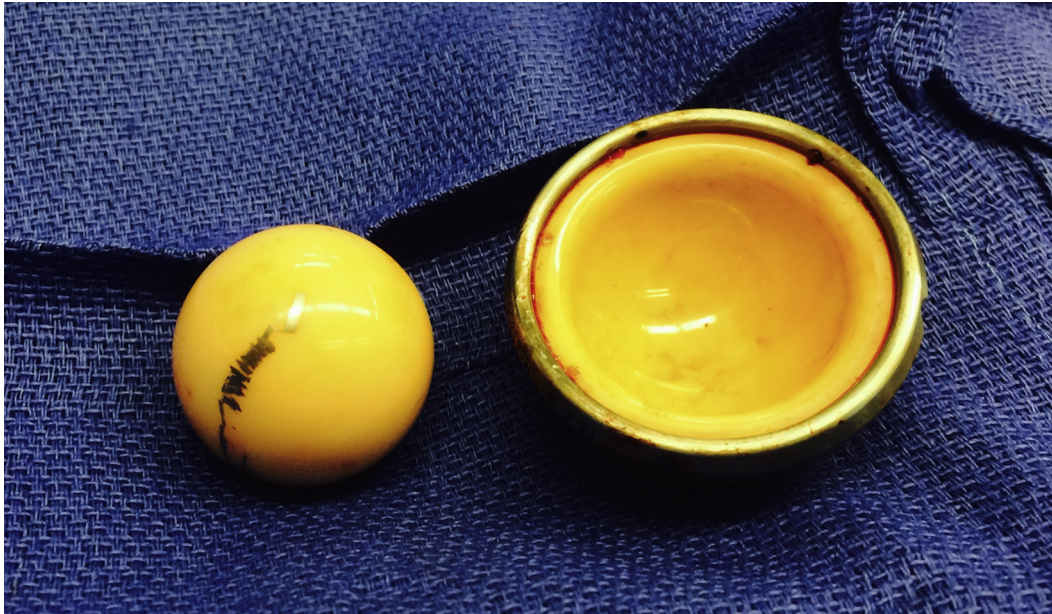
Figure 6. Photograph of removed ceramic components without obvious defects or stripe wear. The “lead pencil” mark was a result of intraoperative dislocation and not present before dislocation.
