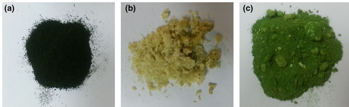
Fig. 2 Images of untreated sample (a), hydrolyzed biomass (b), and residual cell debris (c)
