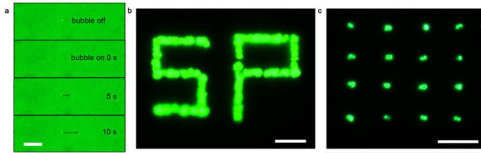
Figure 4. Patterning of PS beads of different sizes on the plasmonic substrates. (a) Time-resolved process for continuous writing of a straight-line pattern of 540 nm PS beads on the AuNIs substrate. (b) Dark-field optical image of the “SP” pattern of 540 nm PS beads. (c) Dark-field optical image of the 4 \times 4 array of 3D hollow structures of 60 nm PS beads. Scale bar: (a) 50 \mu\text{m} ; (b,c) 10 \mu\text{m} .
