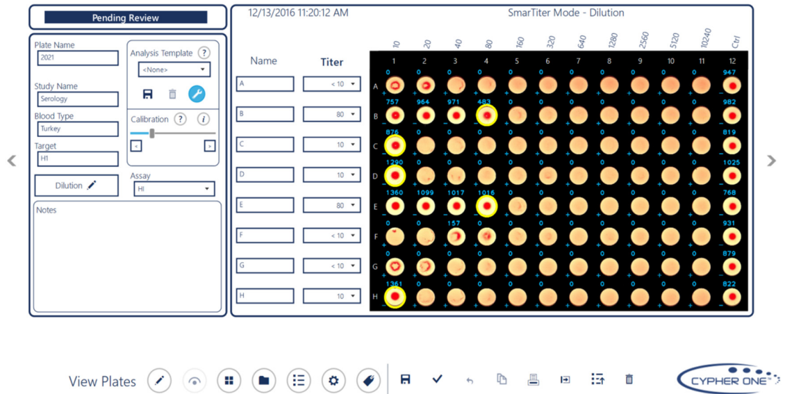
Fig 2. Screen shot of Cypher One user interface. Example HAI plate image within a screen shot of the Cypher One software application. High resolution digital images were captured and titer values determined using an image analysis algorithm within the software. The experimental information, image and resulting titer values are stored as digital records within the system database.
