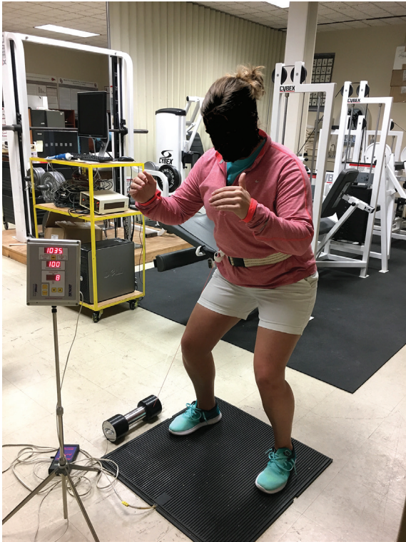
Figure 1. A velocity-sensitive cable can be seen attached near the participant's waist while participant gets ready to do counter-movement jumps on the jump mat with no restriction to their arm movements.
