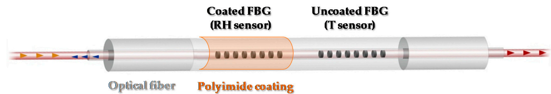
Figure 1. Schematics of the fiber optic thermo-hygrometer.
