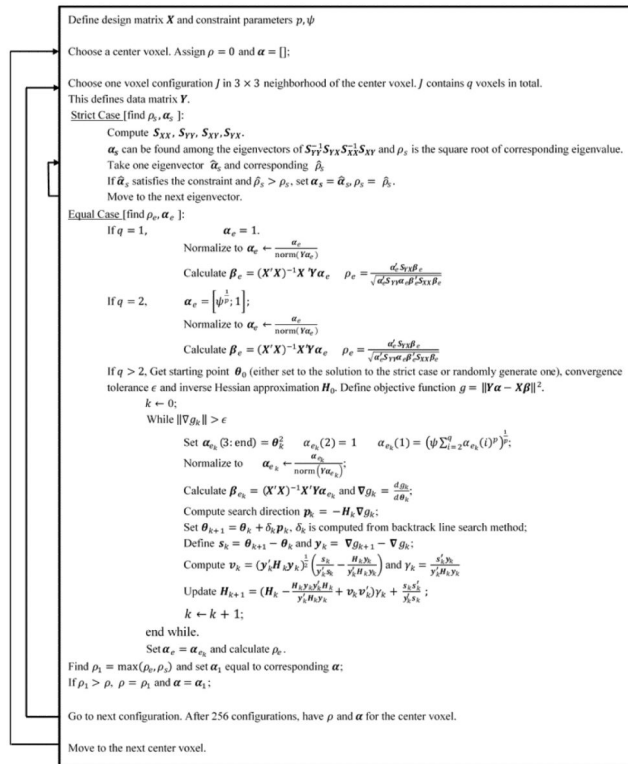
Figure 1. Flow chart of the proposed algorithm in solving the cCCA model considering 256 configurations. All derivatives \nabla g_k are calculated numerically. Note that self-scaling is implemented by parameter \gamma_k .
