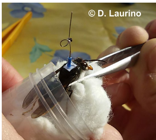
FIGURE 9 Mounting procedure: Once captured, the hornets are put in a Falcon tube, immobilized with a cotton swab and a pair of tweezers, and loaded with the tag, previously mounted on a small paper support with a rubber cylindrical cladding
