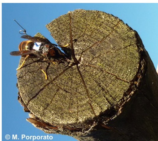
FIGURE 8 "Loop" tag mounted in vertical position on a hornet. To simplify the mounting procedure, the tag was previously glued to a small paper disk and held firm with the help of the external copper wire rubber covering
