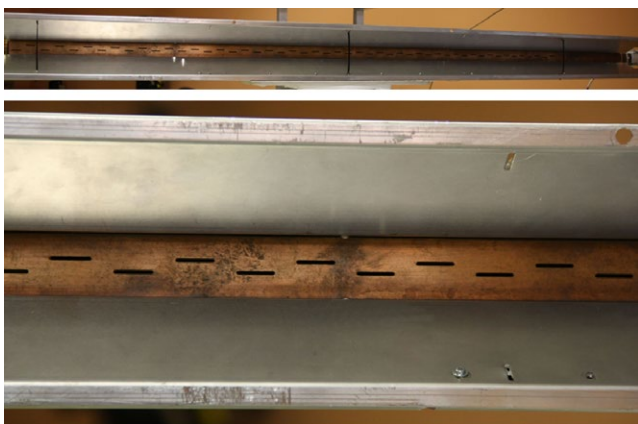
FIGURE 3 New TX vertically polarized slotted waveguide antenna (top) with a detail of the slots (bottom) carved on its surface. The position of the slots with respect to the center of the waveguide and their length allow to choose the amount of power delivered by each radiating element and, eventually, to optimize the radiated field on the azimuthal plane
