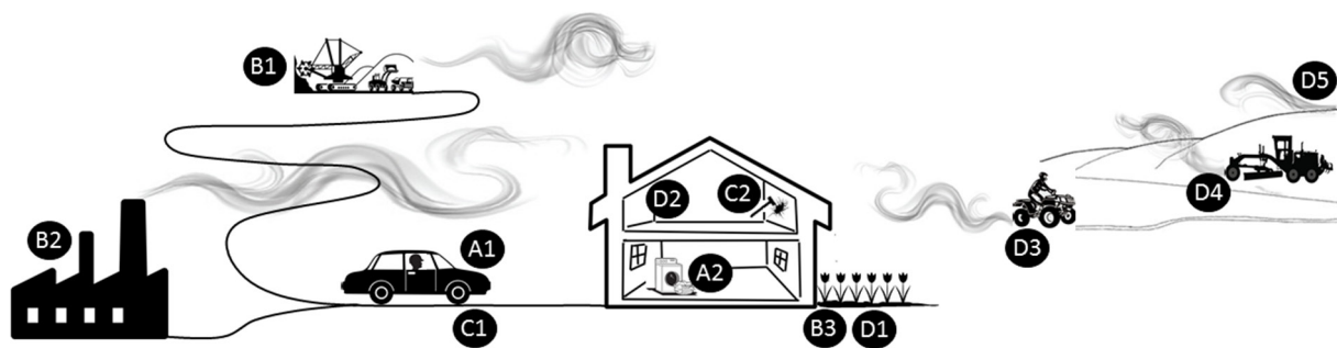
Figure 1 Potential pathways for environmental exposure to asbestos. (A) Para-occupational exposure occurs when asbestos-exposed workers function as vectors for transporting fibers. Household contacts can be exposed in worker vehicles (A1) or through contact with worker clothes or other dust deposits in the home (A2). (B) Environmental exposure from industrial operations. Airborne contamination to communities can be attributed to emissions from nearby mining operations (B1) or asbestos industry (B2). Communities can also be exposed to tailings or asbestos-laden industrial waste materials when used in roadways or soils (B3). (C) Exposure to commercial asbestos-containing products. Asbestos is in numerous products, including automotive brakes (C1) and several housing materials that can be readily disturbed during home maintenance or renovation projects (C2). (D) Naturally occurring asbestos (NOA). In several parts of the world humans have been exposed to asbestos through local use of NOA materials for roads and soil amendments (D1) and as a component in whitewash, stucco or other building materials (D2). Human contact with locations of exposed NOA can result in fiber release through recreational interaction (D3) and development projects (D4). NOA materials can also be released through natural erosion and wind (D5).
