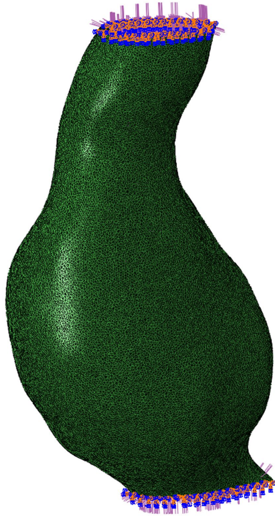
Figure 14. Example of Abaqus model, showing constraints applied on the top and bottom surfaces of the AAA. Definitions of the important surfaces in the model (where loads and boundary conditions are applied) are created by the software and available to the user in the generated input files.
