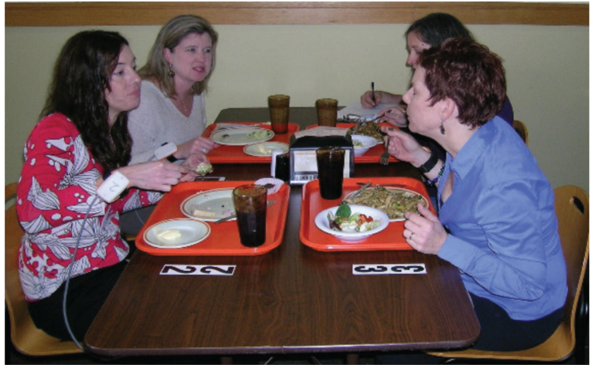
Fig. 1. The table instrumented for data collection. Each participant wore a custom tethered device to track wrist motion.
