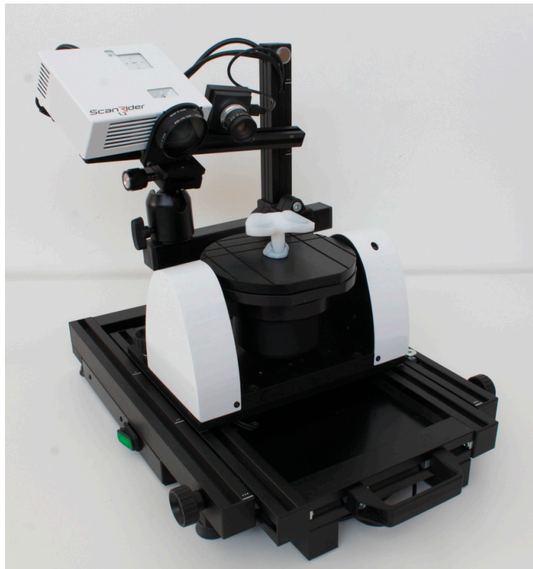
Figure 2. ScanRider 3D, automated metrological optical scanner while scanning a mobile meniscus.
