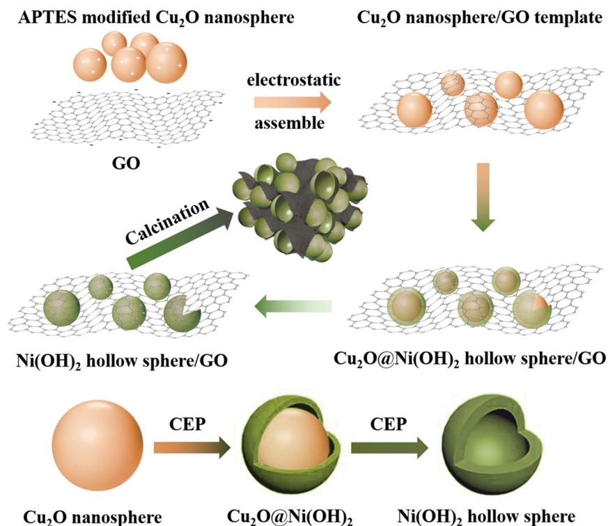
Figure 1. Schematic illustration of the synthesis procedure for 3D NiO hollow sphere/rGO composite. Abbreviations: CEP, coordinating etching and precipitating.
