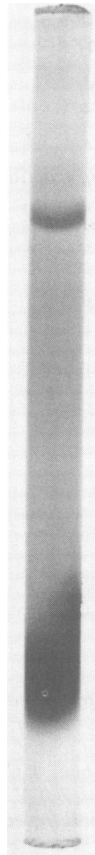
FIG. 3. Polyacrylamide gel electrophoresis of purified equi factor. The origin was at the top, and the anode was at the bottom. See text.
