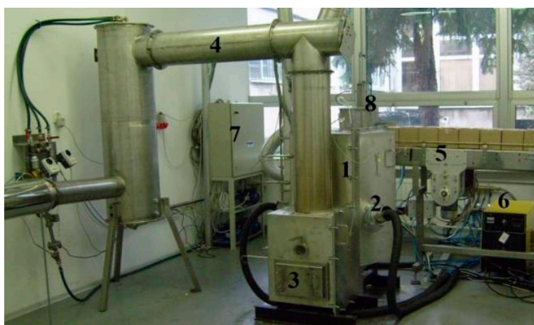
Figure 2. Overview of the laboratory setup: (1) plasma reactor; (2) plasmatron; (3) molten product collection; (4) fumes exhaust–chimney; (5) waste package transporter; (6) plasmatron power supply; (7) PLC-automation and data collection apparatus cabinet; (8) automatic waste package feeder.
