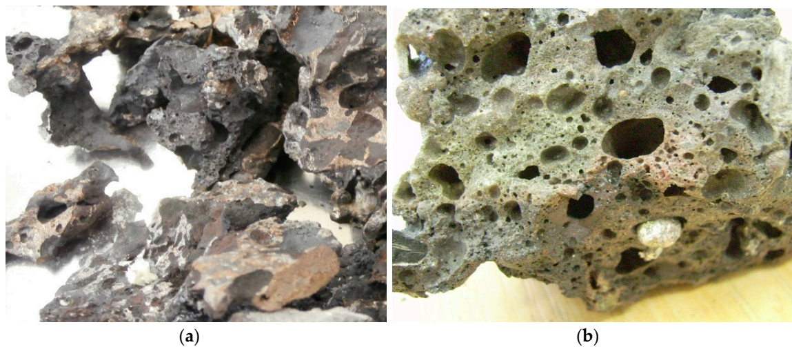
Figure 6. Photograph of separated products—metals (a); and slag (b).
