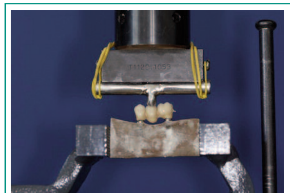
Figure 9 Sample during three point bending test.
