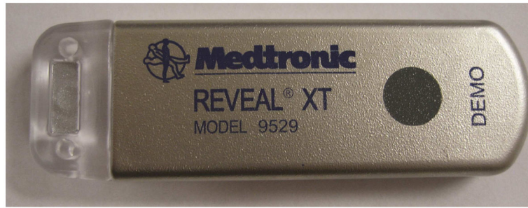
Figure 1. Reveal XT implantable loop recording device
