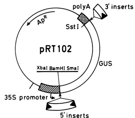
Fig. 2. The plasmid pRT102 used as the source of the wildtype GUS allele. Unique restriction sites used for insertion of I element sequences 5' or 3' of the GUS open reading frame (represented as an open box) are shown. The hatched boxes represent the 35S promoter and polyadenylation sequences. Ap<sup>R</sup> refers to the bacterial  $\beta$ -lactamase gene. I element sequences are represented as in Figure 1.
