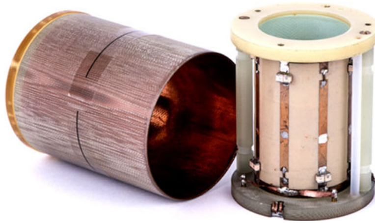
Fig. 1. Birdcage RF coil for ^{35}\text{Cl} in vivo MRI
