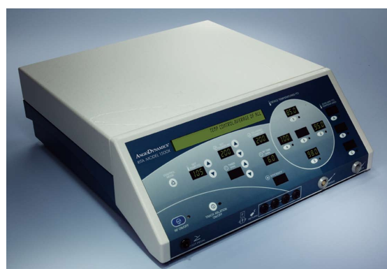
Figure 2 Radiofrequency generator (RITA 1500 X, ANGIODYNAMICS).
