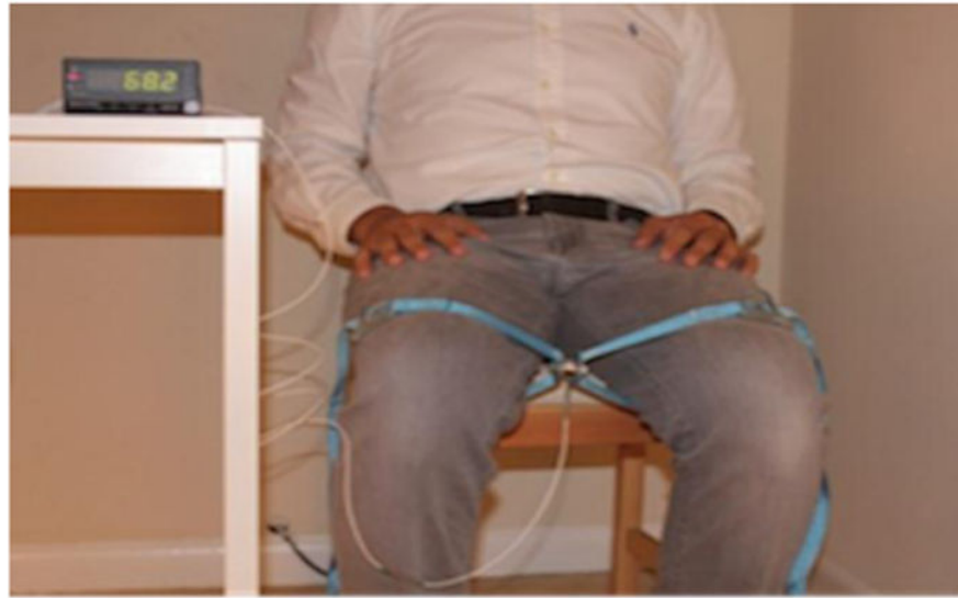
Figure 2. A uni-axial load cell placed between the subject's legs and secured with straps to measure hip abduction muscle strength, which is displayed by the indicator on the table.
