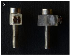
**Fig. 1 a** The clinical simulation device used in this study. **b** Block representative of the teeth attached to the screw
