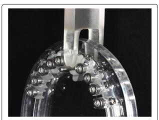
**Fig. 2** Tip of the universal testing machine moving bucco-palatally the acrylic block
