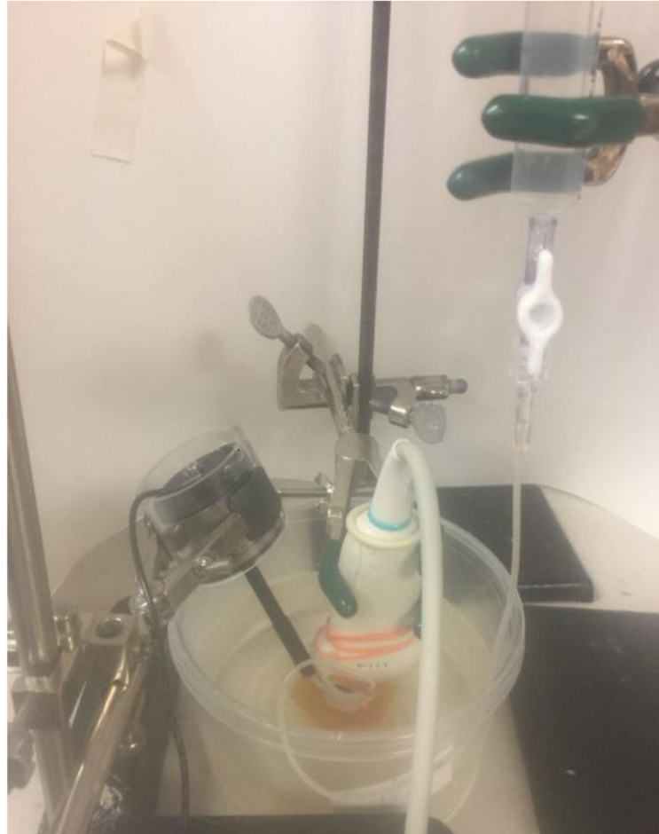
Figure 1. Experimental setup of the USWE system. The shaker was in touch with the limbus region of eye ball to generate a 0.1 second harmonic vibration while an ultrasound probe was placed over the eye ball to measure the wave speed of cornea noninvasively. A butterfly needle was inserted in the vitreous region of the eyeball with the ultrasound imaging guidance. The needle was connected to a syringe filled with water. The IOP was obtained by the water column height of the syringe relative to the water level in the testing container. The IOP was changed from 5 mmHg to 30 mmHg with an interval of 5 mmHg.
