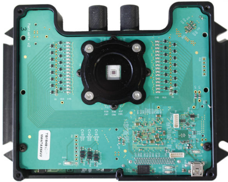
Figure 2. Front view of the detection module, where it is possible to notice the sealed chamber and the entrance window for the light.
