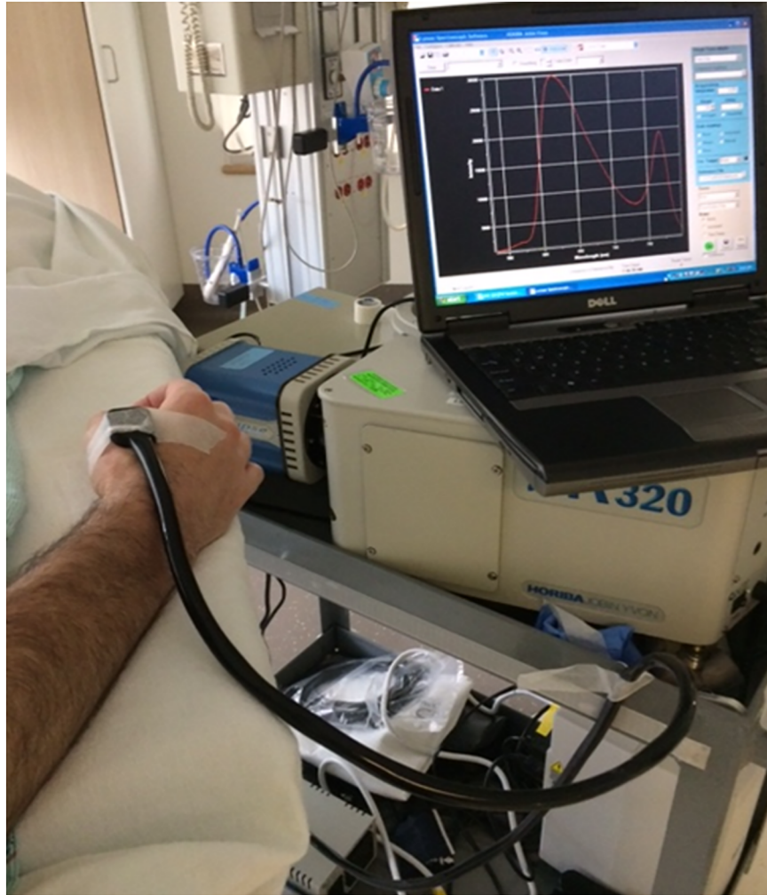
Fig 2. Photograph of the optical probe placed on a subject's hand. The spectrometer and associated equipment is on a mobile cart at the bedside.
