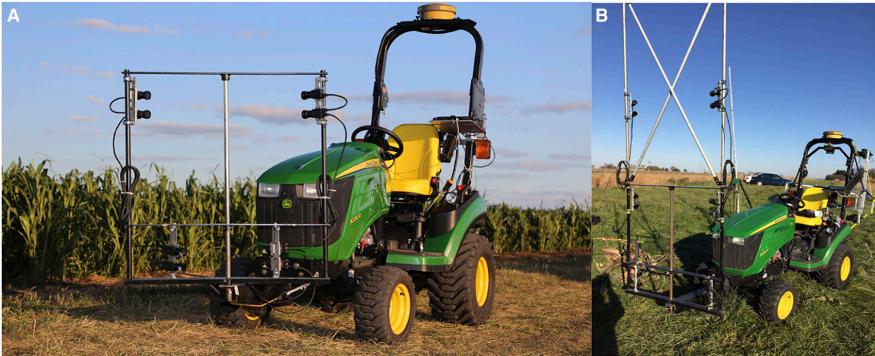
Figure 1. Phenotyping robot (Phenobot) without (A) and with extension rig (B) holding sets of stereo cameras.
