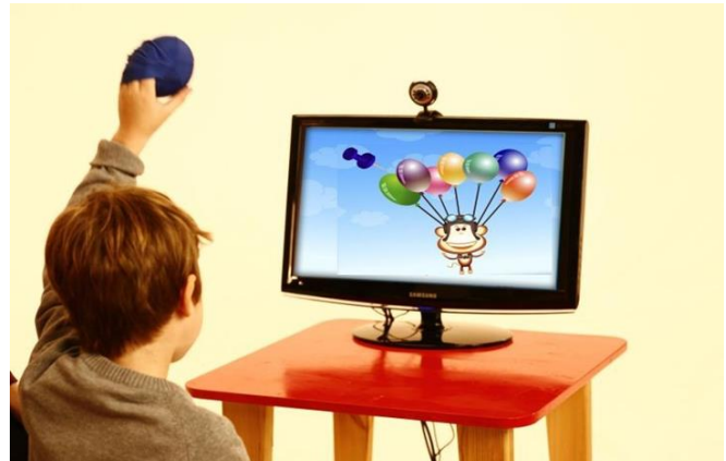
Figure 1. Timocco game set-up. The webcam is tracking the motions of the child by capturing the image of the gaming ball. In this image, the child's goal is to virtually "pop" the balloons with the "push pin," on the screen, which moves in real-time as the child moves his left upper extremity.
