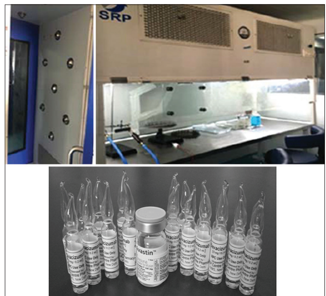
Figure 3: Air curtains and laminar flow-hood facility (Class 10) at our center for sterile dispensing of bevacizumab vial into single dose ampoules
