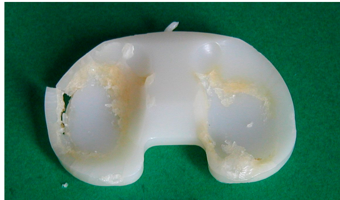
Figure 3. Retrieved polyethylene tibial insert showing severe wear damage, including severe delamination and wear (10 years in vivo ).
