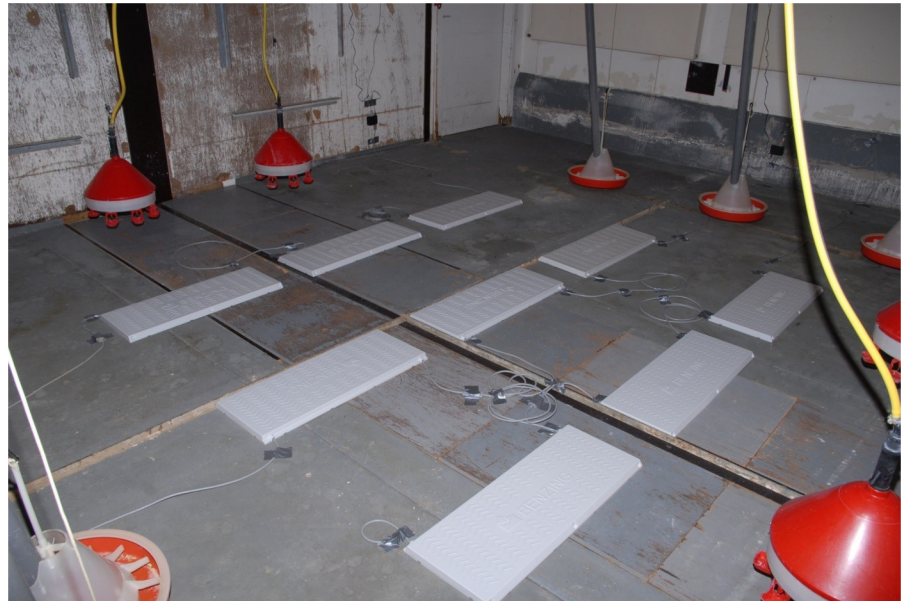
Fig 1. Experimental set up showing the placement of antennas covering the central part of the home pen. A 5 cm layer of cut straw was applied to the floor covering the antennas during the experiment. The recording period was the 11 h light period over five days totalling 55 h.
