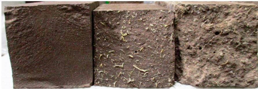
Figure 12. Fracture surface of pristine geopolymer, reinforced with untreated abaca and reinforced with treated abaca.
