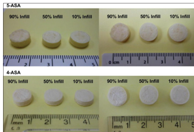
Figure 4: Images of the three-dimensional printed fabricated tablets with different infill percentage. [23] Reprinted with permission
