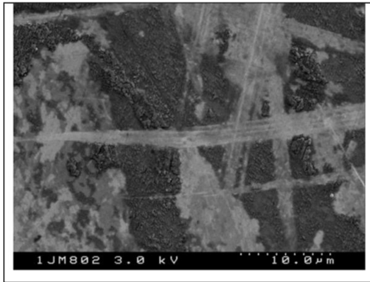
Figure 1. Typical morphology of a McKee-Farrar Hip Joint explant [35]
