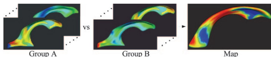
Fig. 3. Concept of statistical significance maps. For two groups of objects, surface distance maps are compared locally, resulting in a map of statistical tests, which displays locations of significant differences between groups.
