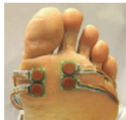
FIGURE 2: Force sensors on the 1st and 2nd MTH used for validation of the estimation algorithm.
