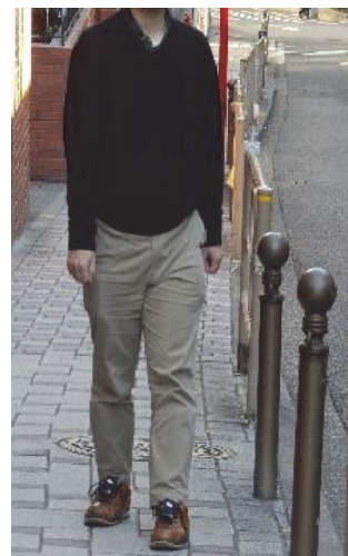
FIGURE 6: Walking measurement for identification of the places where the excessive FL occurs in daily walks. A motion sensor was attached to each shoe.
