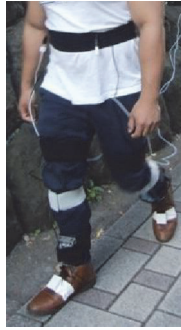
FIGURE 1: Walking measurement for validation of the estimation algorithm. A motion sensor was attached to each of the lower body segment; in addition, 4 force sensors were attached to 1st and 2nd MTH (2 sensors each).
