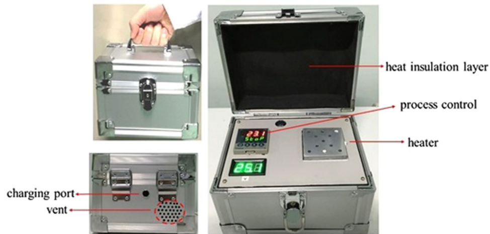
Figure 8. A photograph of the handheld battery-powered heating device. The main components of the handheld battery-powered heating device are a process-controlling module and a metal heater module. There are vents and charging port on the back of the device and a heat insulation layer on the top of the device.
