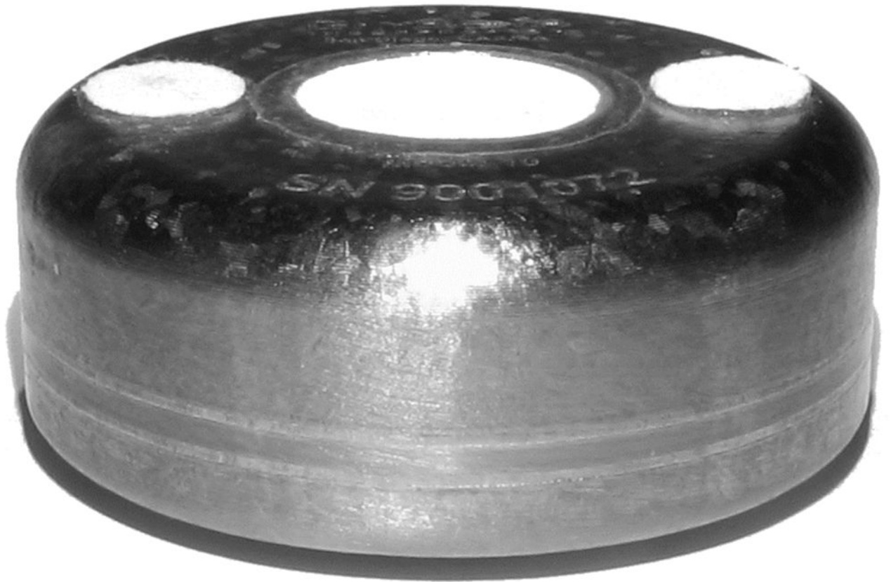
Fig. 1. The glucose sensor/telemetry system implant [9] The implant is 3.4 cm in diameter and 1.5 cm thick.
