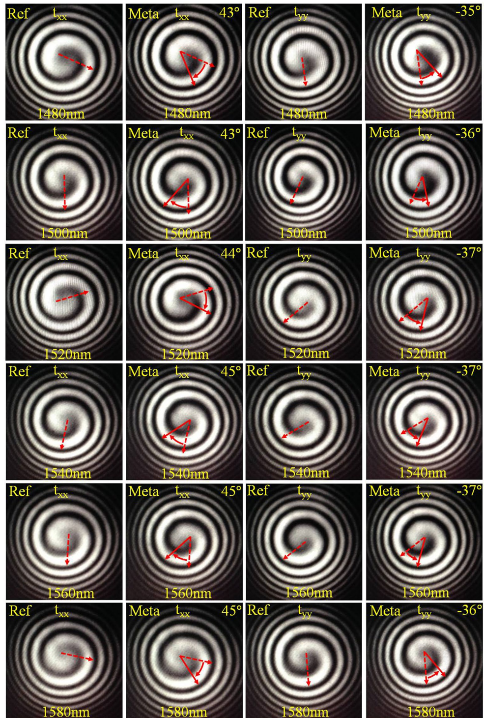
Figure 3. Recorded images of the vortex based spiral interference patterns for optical beam passing through the reference glass substrate (Ref) and the metasurface sample (Meta) under two orthogonal linear polarizations at wavelengths from 1480 nm to 1580 nm with a 20 nm interval. The rotation angles \phi_{xx} and \phi_{yy} of the spiral interference patterns from the metasurface relative to the reference glass substrate are listed.
