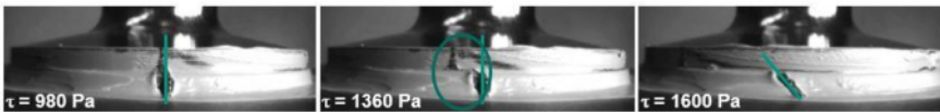
Figure 5. Cutouts from video recordings at varying shear stress. Here using the example of paste A measured with plate roughness R_q = 2 - 4 \mu\text{m} . Please click here to view a larger version of this figure.
