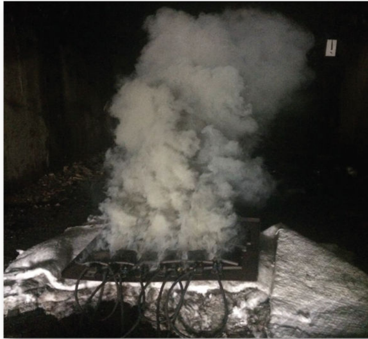
Figure 4. Smoking conveyor belt fire.
