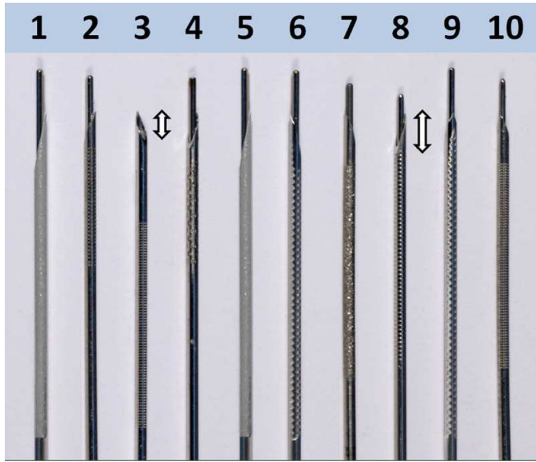
Figure 1. Image of all 10 study needles showing the needle tips (double-headed arrows), shafts, and treated mid shafts to enhance their echogenicity.
