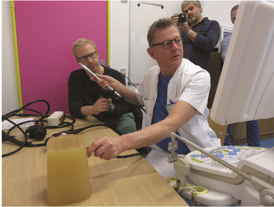
Figure 2. Image showing the bench-top testing setup: a tissue equivalent phantom block and the performing endosonographer (PV).
