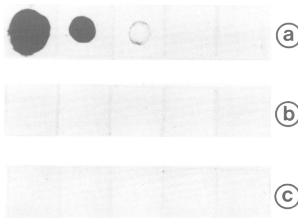
Fig. 1. Immunospot-binding test using monoclonal antibodies with BSP-2 antigen spotted in 1 \mu l volumes and steps of 1:5 dilution in horizontal lanes from left to right. The first spot on the left contains 0.2 \mu g protein. (a) Monoclonal BSP-2 antibody; (b) monoclonal L1 antibody; (c) monoclonal M4 antibody (negative control). All antibodies are derived from rat and used at dilutions of 1:25 (a,b) and 1:10 (c).
