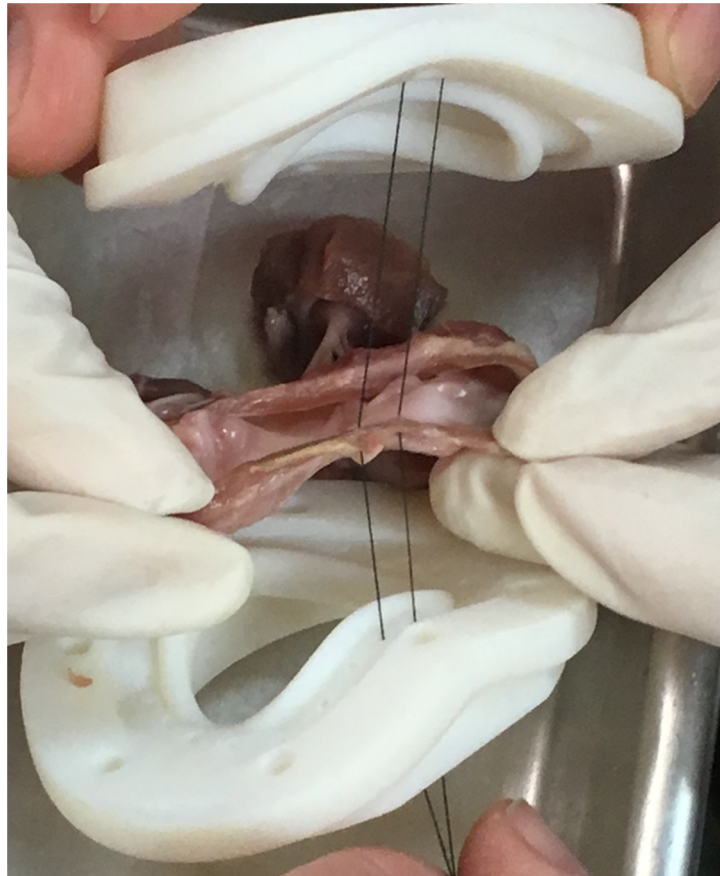
Fig 9. Mounting the mitral valve in the annulus clamp device. For demonstration purposes, the tissue guiding suture is shown without the annulus being wrapped in Dacron.
