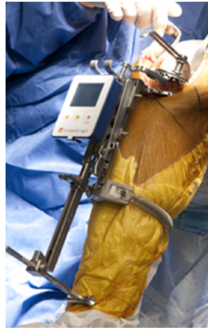
Fig. 1 KneeAlign accelerometer-based knee navigation (OrthoAlign Aliso Viejo, CA) (Courtesy of Seth Jerabek)
