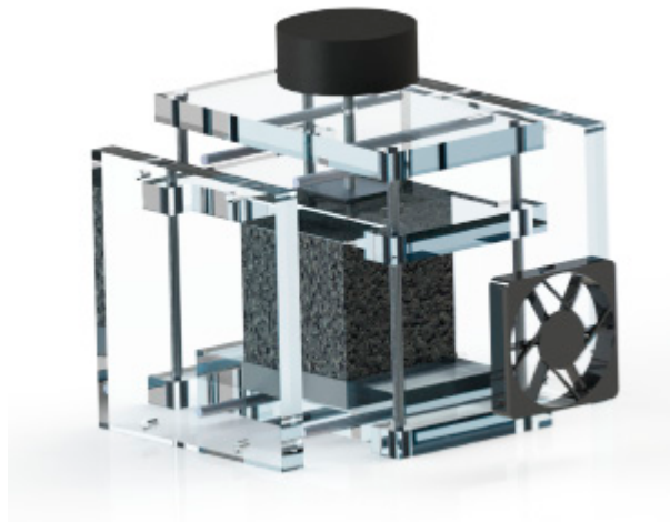
Figure 3. CAD modelling of the experimental set-up for the configuration with load.
