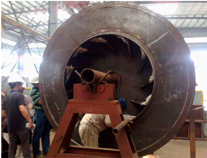
Figure 16. Photograph of the centrifugal compressor with a fully developed blade crack.
